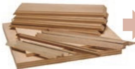
Wood from the Ho tree (Magnolia family) and top-quality Shina plywood is evaluated and dried thoroughly. The parts to be used in the final product are cut out and planed.
