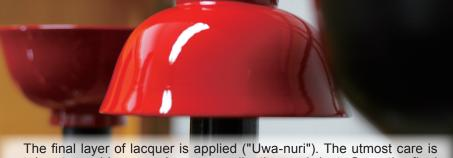
taken to avoid uneven lacquer application and dust. Once the final lacquer application has been completed, the bowl is ready to be dried in a special drying closet. The bowl is turned periodically to ensure even drying.
