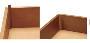
The parts are assembled into a boxshape and "Sumigi" (slender wooden stakes) are placed in the four corners in order to secure the structure. The box is planed to create rounded corners and edges.
